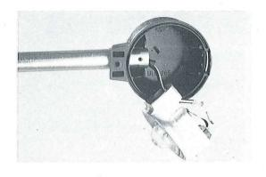
Remove turn signal glass after having removed the screw.
