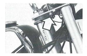
Unscrew the four hex nuts (13 mm wrench size) and remove the clamps.
