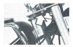
Unscrew the four hex nuts (13 mm wrench size) and remove the clamps.
