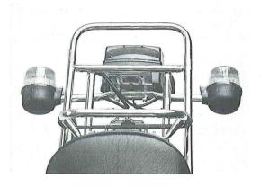
Place turn signal holder from the rear against the taillight and fasten with one each spring lock washer and cap nut.
