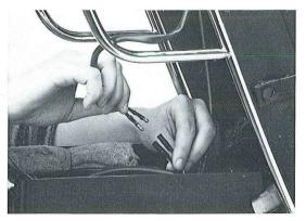
Connect turn signal cables underneath the dual seat to the exposed cable ends of matching color.
