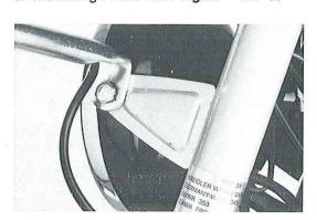
Unscrew headlight fastening screws and fit right and left turn signal holder as shown on the picture.
